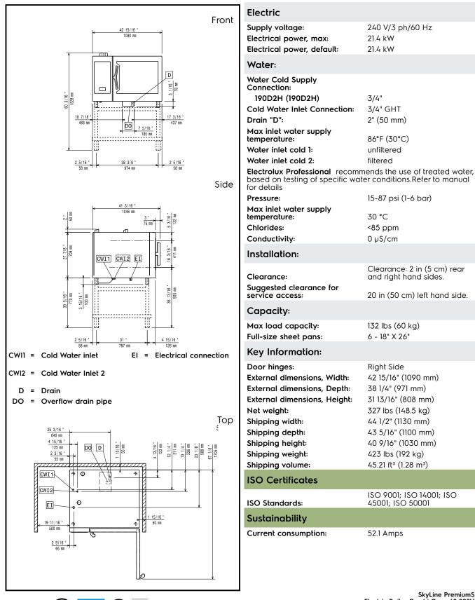
Electric Boiler Combi Oven 62 208V
